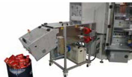
UNLOAD STATION WITH PACKAGE SLITT
