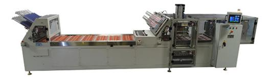
**Starview Packaging Machinery, Inc.** a premier manufacturer of packaging machines is pleased to introduce a newly designed series of Inline Conveyor Heat Sealing Machines for the production of Retail Carded Packaging and Medical / Pharmaceutical Packaging.
