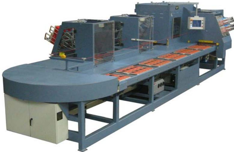
Pictured above is one of three Model BSC II 16-1824 Sixteen-station Carousel Style Fully Automated Blister and Clamshell Sealing Machines we just completed. The machines were specified and sold to a major packager of electronic components by Xpedx, A Division of International Paper.
