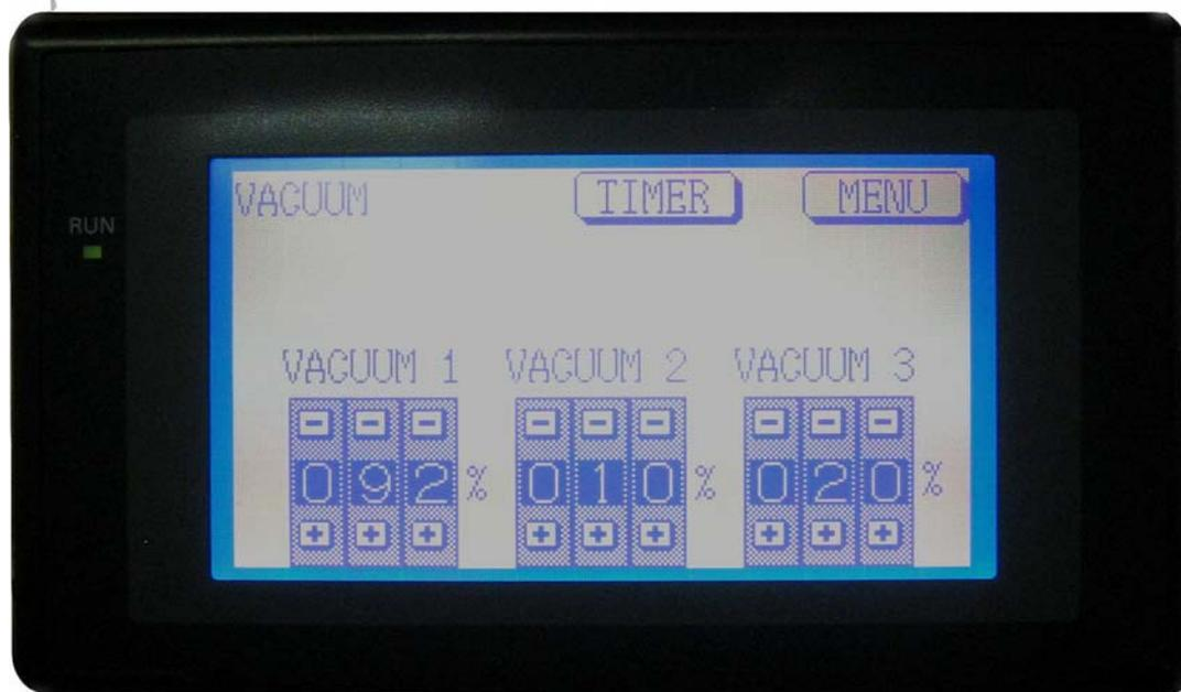
A typical set-up might be Stage 1-a short time and high vacuum speed to evacuate air from under the film quickly, Stage 2 - a longer time and low vacuum speed to reduce webbing and keep film from rupturing around complex parts and finally Stage 3 – a relatively long time and higher vacuum to pull film tightly to the board and provide cooling. Any stage may be skipped by entering zero time.
